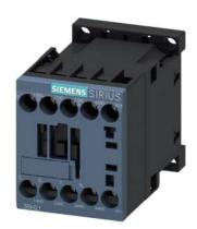
Coupling contactor relay, 3 NO+1 NC 24 V DC, 0.85-1.85\*US with diode integrated Size S00 screw terminal Multi-unit packaging = 40 units
