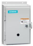
Reversing NEMA contactor Size 1 Three phase full voltage Contactor amp rating 27Amp 3 w 380-440/440-480V 50/60HZ coil Non-combination type Enclosure NEMA type 12 Dust/drip proof for indoors Standard width enclosure
