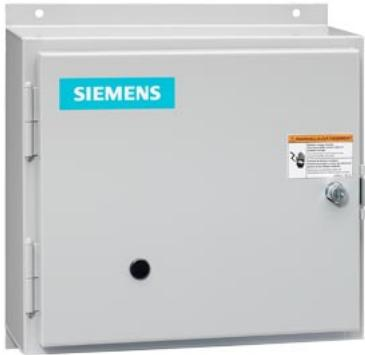
Reversing NEMA contactor Size 0 Three phase full voltage Contactor amp rating 18Amp 3 w 110V 50HZ / 120V 60HZ coil Non-combination type Enclosure NEMA type 12 Dust/drip proof for indoors Standard width enclosure
