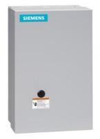
Non-reversing contactor, Size 3 1/2, Three phase full voltage, Contactor amp rating 115A, 3 wire (NO aux included), 220-240/440-480VAC 60Hz coil, Non-combination type, Enclosure NEMA type 1, Indoor general purpose use, Standard width enclosure
