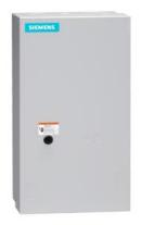
Non-reversing NEMA contactor, Size 3, Three phase full voltage, Contactor amp rating 90A, 3 wire (NO aux included), 240V 50Hz / 277V 60Hz coil, Non-combination type, Enclosure NEMA type 1, Indoor general purpose use, Extra-wide enclosure
