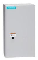
Non-reversing NEMA contactor, Size 3, Three phase full voltage, Contactor amp rating 90A, 3 wire (NO aux included), 110V 50Hz / 120V 60Hz coil, Non-combination type, Enclosure NEMA type 1, Indoor general purpose use, Extra-wide enclosure
