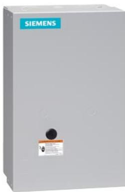
Non-reversing NEMA contactor, Size 3, Three phase full voltage, Contactor amp rating 90A, 3 wire (NO aux included), 208VAC 60Hz coil, Non-combination type, Enclosure NEMA type 1, Indoor general purpose use, Standard width enclosure
