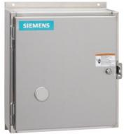
Non-reversing contactor, Size 2 1/2, Three phase full voltage, Contactor amp rating 60A, 3 wire (NO aux included), 110V 50Hz / 120V 60Hz coil, Non-combination type, Encl NEMA type 4X 304 S-Steel, Water/dust tight noncorrosive, Extra-wide enclosure
