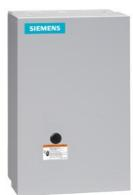
Non-reversing contactor, Size 2 1/2, Three phase full voltage, Contactor amp rating 60A, 3 wire (NO aux included), 110-120/220-240VAC 60Hz coil, Non-combination type, Enclosure NEMA type 1, Indoor general purpose use, Extra-wide enclosure
