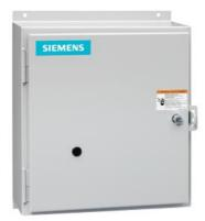
Non-reversing contactor, Size 2 1/2, Three phase full voltage, Contactor amp rating 60A, 3 wire (NO aux included), 110V 50Hz / 120V 60Hz coil, Non-combination type, Enclosure NEMA type 12, Dust/drip proof for indoors, Extra-wide enclosure
