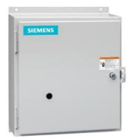
Non-reversing contactor, Size 2 1/2, Three phase full voltage, Contactor amp rating 60A, 3 wire (NO aux included), 110-120/220-240VAC 60Hz coil, Non-combination type, Enclosure NEMA type 12, Dust/drip proof for indoors, Extra-wide enclosure
