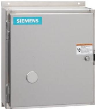
Non-reversing NEMA contactor, Size 2, Three phase full voltage, Contactor amp rating 45A, 3 wire (NO aux included), 380-440/440-480V 50/60Hz coil, Non-combination type, Encl NEMA type 4X 304 S-Steel, Water/dust tight noncorrosive, Extra-wide enclosure
