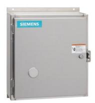
Non-reversing NEMA contactor, Size 2, Three phase full voltage, Contactor amp rating 45A, 3 wire (NO aux included), 220-240/440-480VAC 60Hz coil, Non-combination type, Encl NEMA type 4X 304 S-Steel, Water/dust tight noncorrosive, Extra-wide enclosure
