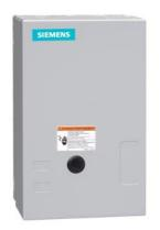
Non-reversing NEMA contactor, Size 2, Three phase full voltage, Contactor amp rating 45A, 3 wire (NO aux included), 240V 50Hz / 277V 60Hz coil, Non-combination type, Enclosure NEMA type 1, Indoor general purpose use, Extra-wide enclosure
