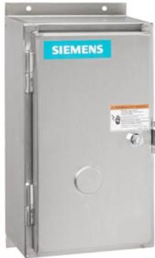
Non-reversing NEMA contactor, Size 2, Three phase full voltage, Contactor amp rating 45A, 3 wire (NO aux included), 220-240/440-480VAC 60Hz coil, Non-combination type, Encl NEMA type 4X 304 S-Steel, Water/dust tight noncorrosive, Standard width enclosure
