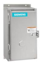
Non-reversing NEMA contactor, Size 2, Three phase full voltage, Contactor amp rating 45A, 3 wire (NO aux included), 110-120/220-240VAC 60Hz coil, Non-combination type, Encl NEMA type 4X 304 S-Steel, Water/dust tight noncorrosive, Standard width enclosure
