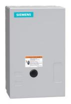
Non-reversing NEMA contactor, Size 2, Three phase full voltage, Contactor amp rating 45A, 3 wire (NO aux included), 208VAC 60Hz coil, Non-combination type, Enclosure NEMA type 1, Indoor general purpose use, Standard width enclosure
