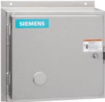
Non-reversing contactor, Size 1 3/4, Three phase full voltage, Contactor amp rating 40A, 3 wire (NO aux included), 24VAC 50-60Hz coil, Non-combination type, Encl NEMA type 4X 304 S-Steel, Water/dust tight noncorrosive, Extra-wide enclosure
