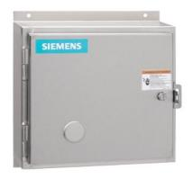
Non-reversing contactor, Size 1 3/4, Three phase full voltage, Contactor amp rating 40A, 3 wire (NO aux included), 110-120/220-240VAC 60Hz coil, Non-combination type, Encl NEMA type 4X 304 S-Steel, Water/dust tight noncorrosive, Extra-wide enclosure
