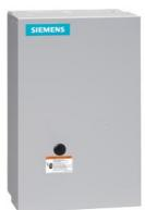
Non-reversing contactor, Size 1 3/4, Three phase full voltage, Contactor amp rating 40A, 3 wire (NO aux included), 24VAC 50-60Hz coil, Non-combination type, Enclosure NEMA type 1, Indoor general purpose use, Extra-wide enclosure
