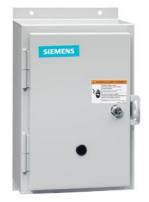
Non-reversing contactor, Size 1 3/4, Three phase full voltage, Contactor amp rating 40A, 3 wire (NO aux included), 24VAC 50-60Hz coil, Non-combination type, Enclosure NEMA type 12, Dust/drip proof for indoors, Extra-wide enclosure
