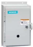
Non-reversing contactor, Size 1 3/4, Three phase full voltage, Contactor amp rating 40A, 3 wire (NO aux included), 380-440/440-480V 50/60Hz coil, Non-combination type, Enclosure NEMA type 12, Dust/drip proof for indoors, Extra-wide enclosure
