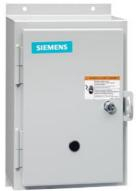
Non-reversing contactor, Size 1 3/4, Three phase full voltage, Contactor amp rating 40A, 3 wire (NO aux included), 208VAC 60Hz coil, Non-combination type, Enclosure NEMA type 12, Dust/drip proof for indoors, Extra-wide enclosure
