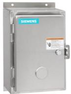
Non-reversing contactor, Size 1 3/4, Three phase full voltage, Contactor amp rating 40A, 3 wire (NO aux included), 110V 50Hz / 120V 60Hz coil, Non-combination type, Encl NEMA type 4X 304 S-Steel, Water/dust tight noncorrosive, Standard width enclosure
