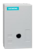
Non-reversing contactor, Size 1 3/4, Three phase full voltage, Contactor amp rating 40A, 3 wire (NO aux included), 24VAC 50-60Hz coil, Non-combination type, Enclosure NEMA type 1, Indoor general purpose use, Standard width enclosure
