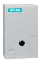
Non-reversing contactor, Size 1 3/4, Three phase full voltage, Contactor amp rating 40A, 3 wire (NO aux included), 550/575-600 50/60Hz coil, Non-combination type, Enclosure NEMA type 1, Indoor general purpose use, Standard width enclosure
