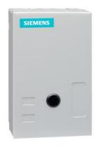
Non-reversing contactor, Size 1 3/4, Three phase full voltage, Contactor amp rating 40A, 3 wire (NO aux included), 220-240/440-480VAC 60Hz coil, Non-combination type, Enclosure NEMA type 1, Indoor general purpose use, Standard width enclosure
