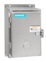
Non-reversing contactor, Size 1 3/4, 4 power poles, Contactor amp rating 40A, 3 wire (NO aux included), 110V 50Hz / 120V 60Hz coil, Non-combination type, Encl NEMA type 4X 304 S-Steel, Water/dust tight noncorrosive, Standard width enclosure
