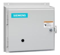
Non-reversing contactor, Size 1 3/4, 4 power poles, Contactor amp rating 40A, 3 wire (NO aux included), 240V 50Hz / 277V 60Hz coil, Non-combination type, Enclosure NEMA type 12, Dust/drip proof for indoors, Standard width enclosure
