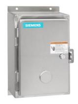
Non-reversing contactor, Size 1P, Single phase full voltage, Contactor amp rating 35A, 3 wire (NO aux included), 24VAC 50-60Hz coil, Non-combination type, Encl NEMA type 4X 304 S-Steel, Water/dust tight noncorrosive, Standard width enclosure
