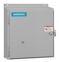
Non-reversing contactor, Size 1P, Single phase full voltage, Contactor amp rating 35A, 3 wire (NO aux included), 110V 50Hz / 120V 60Hz coil, Non-combination type, Encl. NEMA type 4X fiberglass, Water/dust tight noncorrosive, Standard width enclosure
