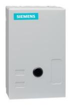
Non-reversing contactor, Size 1P, Single phase full voltage, Contactor amp rating 35A, 3 wire (NO aux included), 110V 50Hz / 120V 60Hz coil, Non-combination type, Enclosure NEMA type 1, Indoor general purpose use, Standard width enclosure
