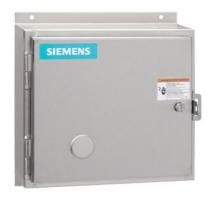
Non-reversing NEMA contactor, Size 1, Three phase full voltage, Contactor amp rating 27A, 3 wire (NO aux included), 240V 50Hz / 277V 60Hz coil, Non-combination type, Encl NEMA type 4X 304 S-Steel, Water/dust tight noncorrosive, Extra-wide enclosure
