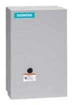
Non-reversing NEMA contactor, Size 1, Three phase full voltage, Contactor amp rating 27A, 3 wire (NO aux included), 208VAC 60Hz coil, Non-combination type, Enclosure NEMA type 1, Indoor general purpose use, Extra-wide enclosure
