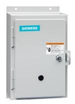
Non-reversing NEMA contactor, Size 1, Three phase full voltage, Contactor amp rating 27A, 3 wire (NO aux included), 24VAC 50-60Hz coil, Non-combination type, Enclosure NEMA type 12, Dust/drip proof for indoors, Extra-wide enclosure
