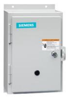
Non-reversing NEMA contactor, Size 1, Three phase full voltage, Contactor amp rating 27A, 3 wire (NO aux included), 190-220/220-240V 50/60Hz coil, Noncombination type, Enclosure NEMA type 12, Dust/drip proof for indoors, Extra-wide enclosure
