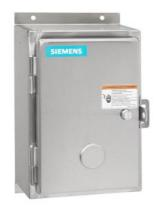
Non-reversing NEMA contactor, Size 1, 4 power poles, Contactor amp rating 27A, 3 wire (NO aux included), 110V 50Hz / 120V 60Hz coil, Non-combination type, Encl NEMA type 4X 304 S-Steel, Water/dust tight noncorrosive, Standard width enclosure
