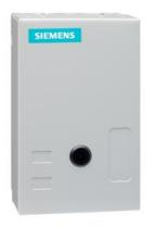
Non-reversing NEMA contactor, Size 1, 4 power poles, Contactor amp rating 27A, 3 wire (NO aux included), 240V 50Hz / 277V 60Hz coil, Non-combination type, Enclosure NEMA type 1, Indoor general purpose use, Standard width enclosure
