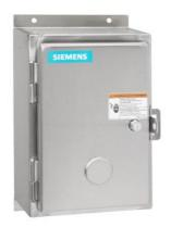
Non-reversing NEMA contactor, Size 1, Single phase full voltage, Contactor amp rating 27A, 3 wire (NO aux included), 110-120/220-240VAC 60Hz coil, Non-combination type, Encl NEMA type 4X 304 S-Steel, Water/dust tight noncorrosive, Standard width enclosure
