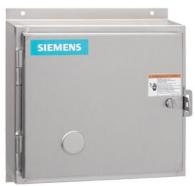
Non-reversing NEMA contactor, Size 0, Three phase full voltage, Contactor amp rating 18A, 3 wire (NO aux included), 110V 50Hz / 120V 60Hz coil, Noncombination type, Encl NEMA type 4X 304 S-Steel, Water/dust tight noncorrosive, Extra-wide enclosure
