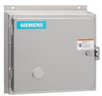
Non-reversing NEMA contactor, Size 0, Three phase full voltage, Contactor amp rating 18A, 3 wire (NO aux included), 208VAC 60Hz coil, Non-combination type, Encl NEMA type 4X 304 S-Steel, Water/dust tight noncorrosive, Extra-wide enclosure
