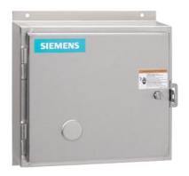
Non-reversing NEMA contactor, Size 0, Three phase full voltage, Contactor amp rating 18A, 3 wire (NO aux included), 110-120/220-240VAC 60Hz coil, Non-combination type, Encl NEMA type 4X 304 S-Steel, Water/dust tight noncorrosive, Extra-wide enclosure
