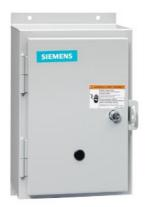
Non-reversing NEMA contactor, Size 0, Three phase full voltage, Contactor amp rating 18A, 3 wire (NO aux included), 240V 50Hz / 277V 60Hz coil, Non-combination type, Enclosure NEMA type 12, Dust/drip proof for indoors, Extra-wide enclosure
