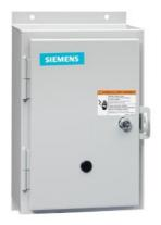
Non-reversing NEMA contactor, Size 0, Three phase full voltage, Contactor amp rating 18A, 3 wire (NO aux included), 24VAC 50-60Hz coil, Non-combination type, Enclosure NEMA type 12, Dust/drip proof for indoors, Extra-wide enclosure
