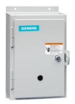
Non-reversing NEMA contactor, Size 0, Three phase full voltage, Contactor amp rating 18A, 3 wire (NO aux included), 208VAC 60Hz coil, Non-combination type, Enclosure NEMA type 12, Dust/drip proof for indoors, Extra-wide enclosure
