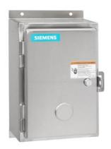
Non-reversing NEMA contactor, Size 0, Three phase full voltage, Contactor amp rating 18A, 3 wire (NO aux included), 110-120/220-240VAC 60Hz coil, Non-combination type, Encl NEMA type 4X 304 S-Steel, Water/dust tight noncorrosive, Standard width enclosure
