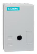
Non-reversing NEMA contactor, Size 0, Three phase full voltage, Contactor amp rating 18A, 3 wire (NO aux included), 110V 50Hz / 120V 60Hz coil, Non-combination type, Enclosure NEMA type 1, Indoor general purpose use, Standard width enclosure
