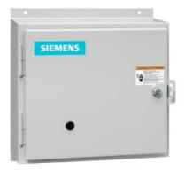
Non-reversing NEMA contactor, Size 0, Three phase full voltage, Contactor amp rating 18A, 3 wire (NO aux included), 220-240/440-480VAC 60Hz coil, Non-combination type, Enclosure NEMA type 12, Dust/drip proof for indoors, Standard width enclosure
