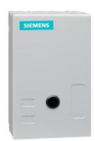
Non-reversing NEMA contactor, Size 0, 4 power poles, Contactor amp rating 18A, 3 wire (NO aux included), 24VAC 50-60Hz coil, Non-combination type, Enclosure NEMA type 1, Indoor general purpose use, Standard width enclosure
