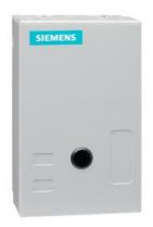
Non-reversing NEMA contactor, Size 0, 4 power poles, Contactor amp rating 18A, 3 wire (NO aux included), 190-220/220-240V 50/60Hz coil, Non-combination type, Enclosure NEMA type 1, Indoor general purpose use, Standard width enclosure
